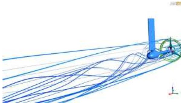
Figure 1: Simulation of an axial rotor turbine. Results will be compared to flume tank experiments.
