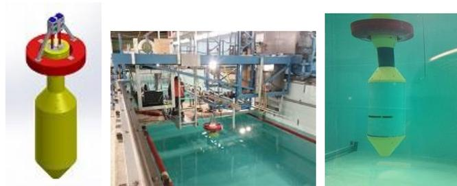
*Images of UVic's experimental WEC. From left to right: Snapshot of the CAD model. View of the WEC mounted in the test tank. View from below the water of the WEC mounted in the test tank.*
