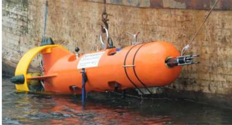
*Figure caption: Recovery of the Nemo turbulence mooring after a five-day deployment in Grand Passage, NS. Turbulence probes are visible protruding from the nose section of the float. Photo by Greg Trowse.*
